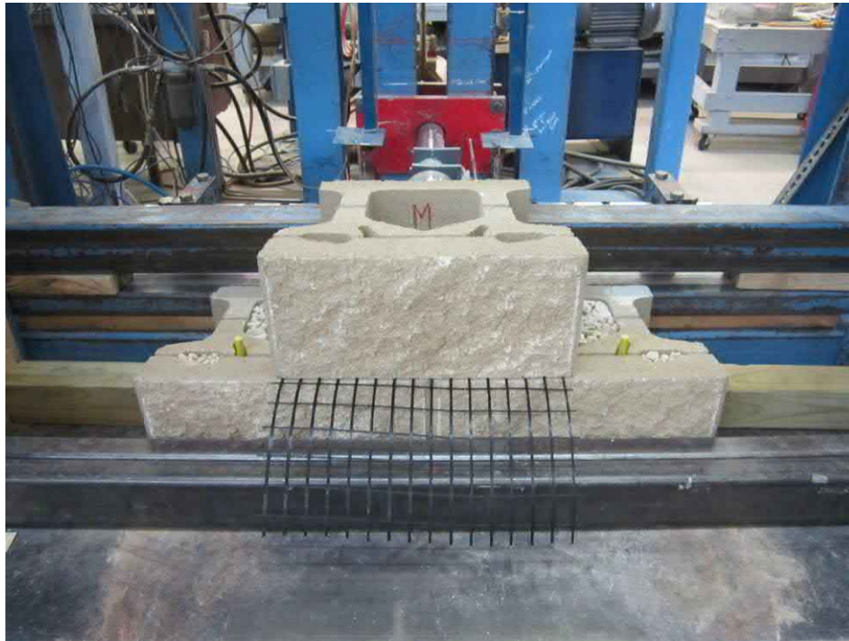
Figure 7: Photograph of a Keystone Compac 3 block centered above the geogrid and the two underlying blocks.
