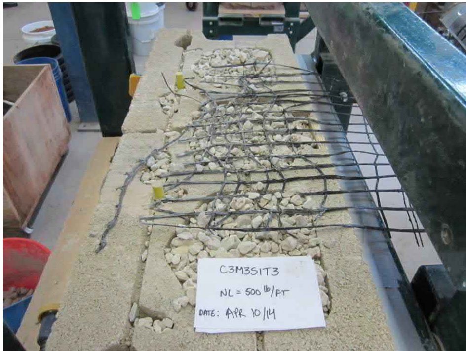
Figure 15: Another photograph of the exhumed grid specimen from Test 1.
