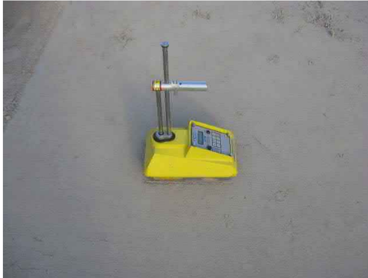
Figure D-3. The density of the compacted soil is measured with a nuclear density gauge.
