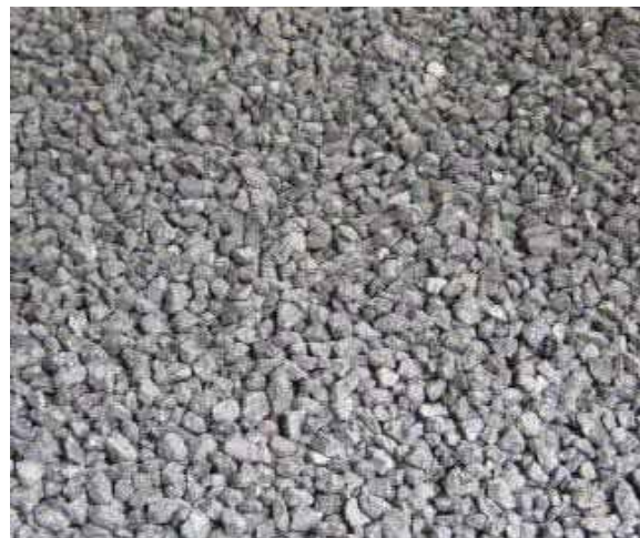
Figure E-2. ISO/EN 10722, laboratory installation damage aggregate.
