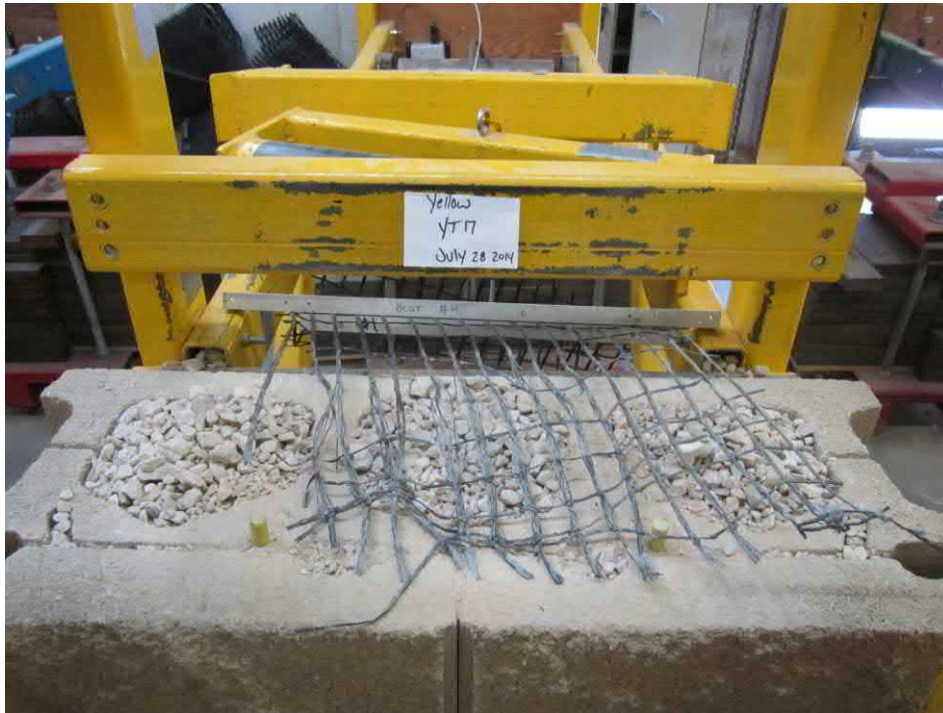
Figure 16: Photograph of exhumed grid specimen from Test 5 of Sustained Load Testing (Normal Load = 1000 lb/ft).
