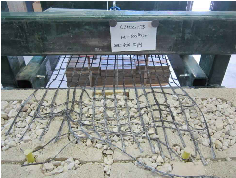
Figure 14: Photograph of exhumed grid specimen from Test 1 of Sustained Load Testing (Normal Load = 500 lb/ft).
