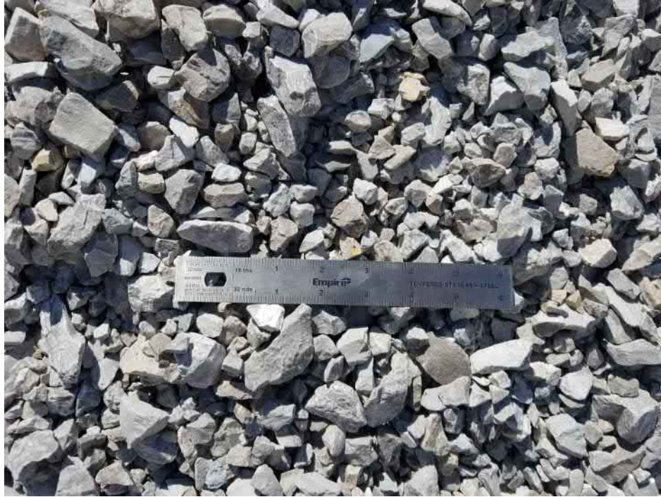
Figure 4-4. Installation damage 57 stone test aggregate.
