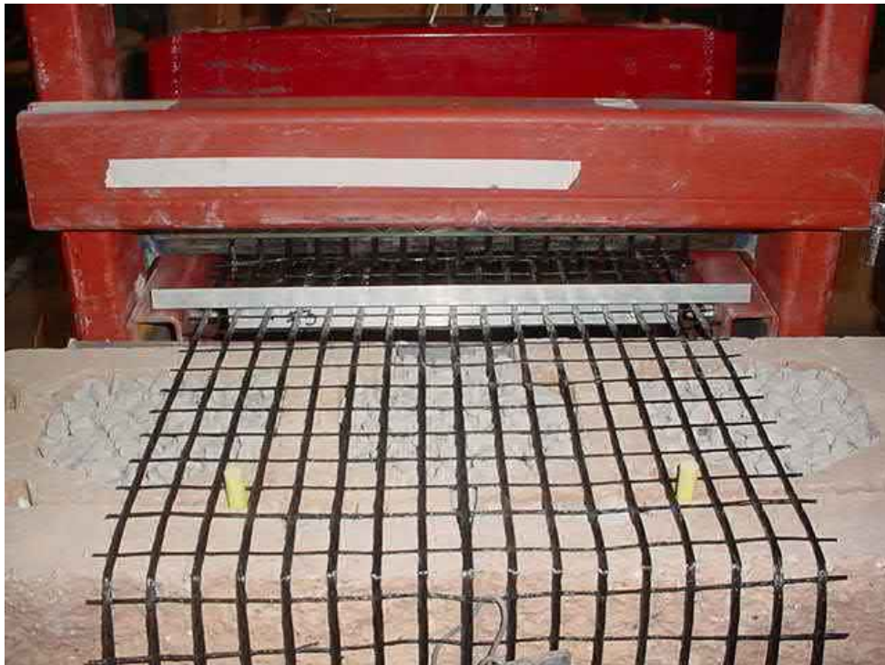
Figure 5: Photograph of the geogrid placed flat over the two bottom blocks.
