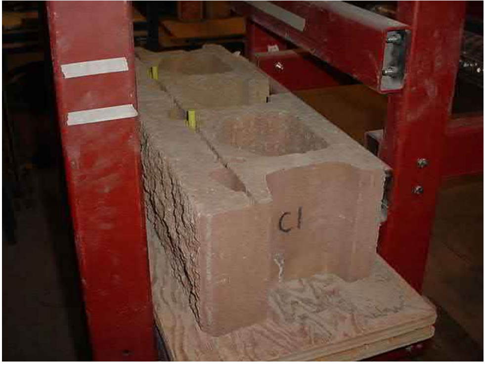
Figure 1: Photograph of a Keystone Compac 3 modular block with fiberglass pins.
