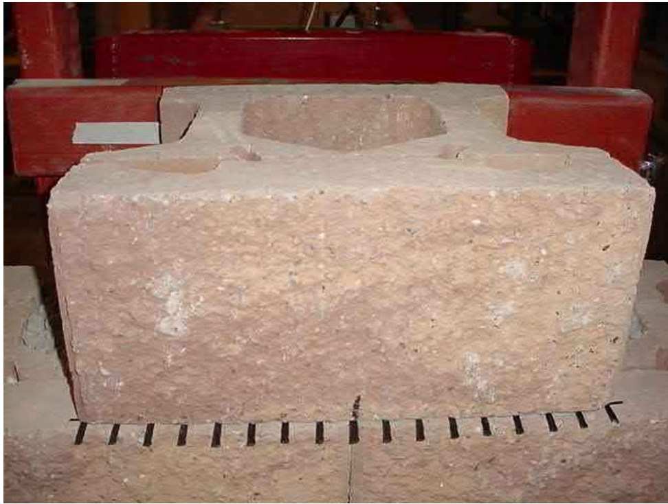
Figure 6: Photograph of a Keystone Compac 3 block centered above the geogrid and the two underlying blocks.
