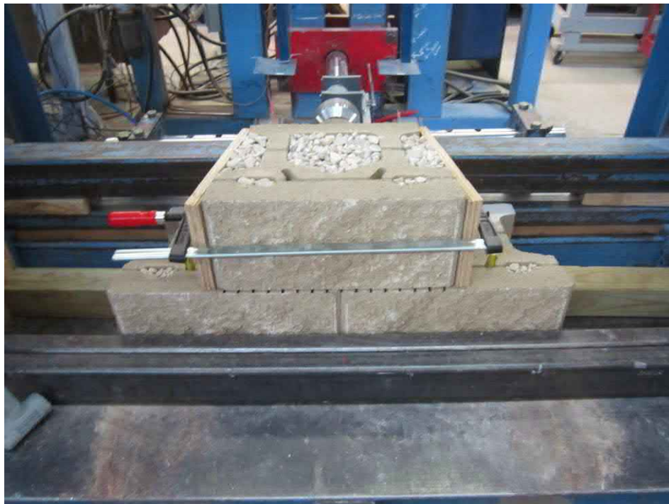
Figure 8: Photograph showing the infill of the top block and containment barriers.
