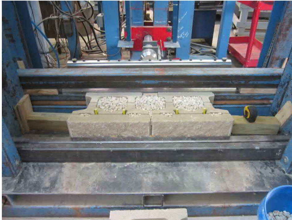
Figure 5: Photograph of the bottom row of blocks and granular fill.
