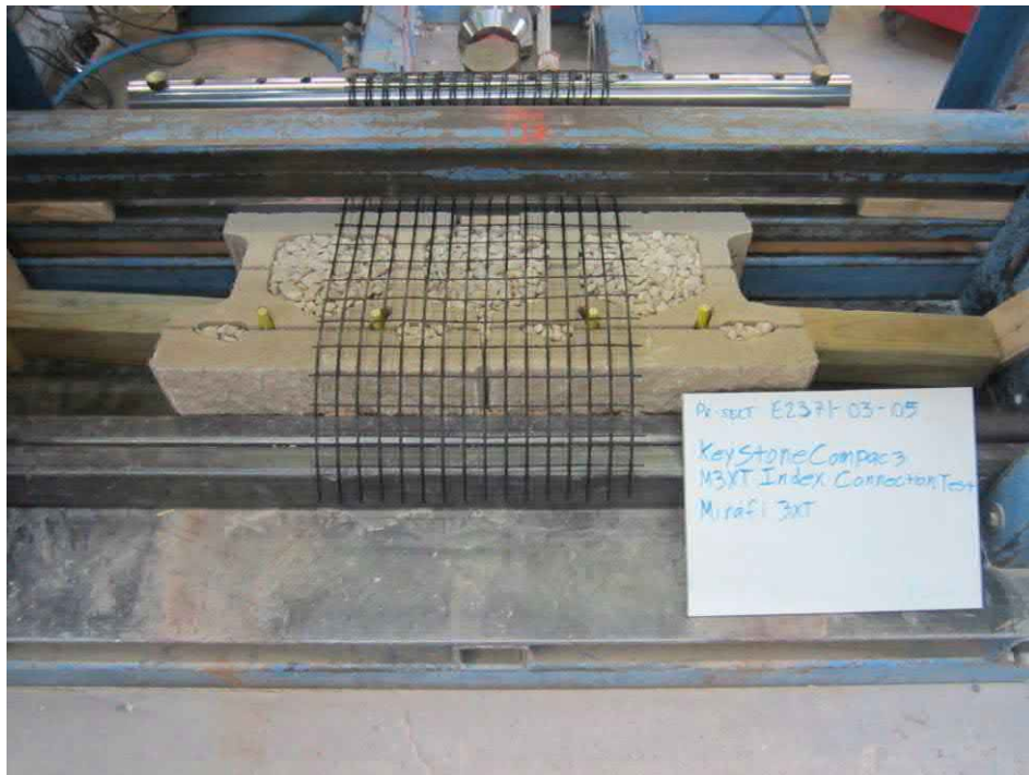
Figure 6: Photograph of the geogrid placed flat over the two bottom blocks.
