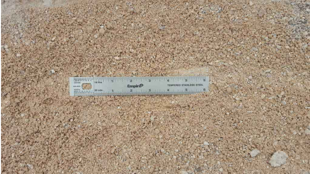
Figure 4-5. Installation damage Type 3 test aggregate.
