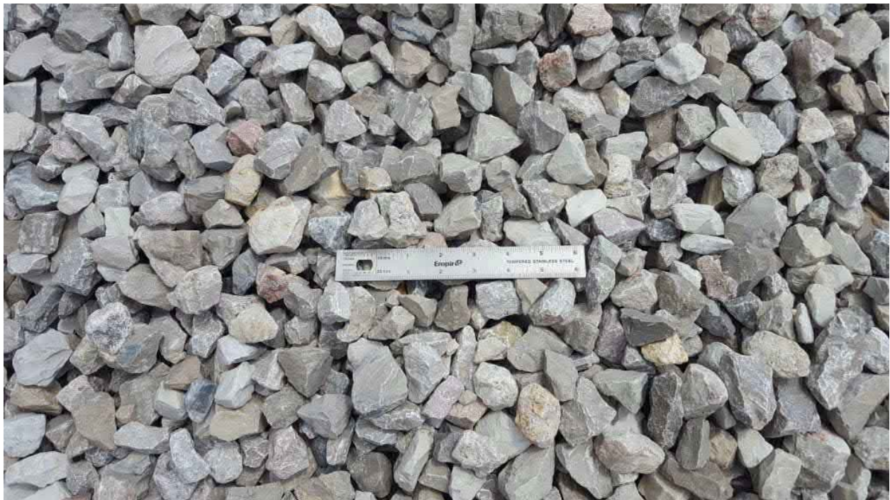
Figure 4-2. Installation damage Type 1 test aggregate.
