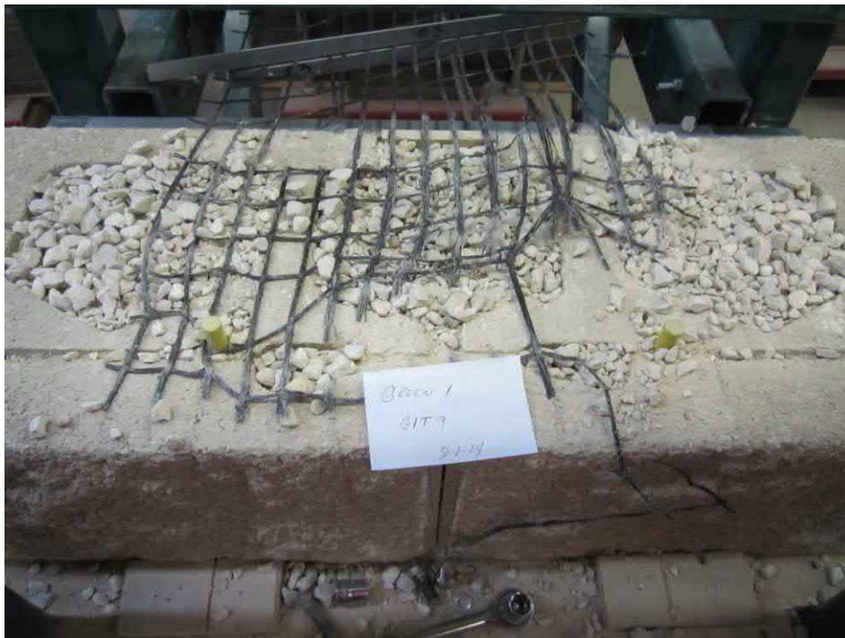
Figure 17: Photograph of exhumed grid specimen from Test 7 of Sustained Load Testing (Normal Load = 2000 lb/ft).
