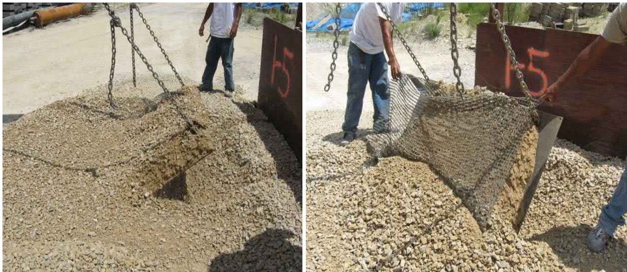
Figure D-4. The steel plates are tilted to facilitate exhumation.
