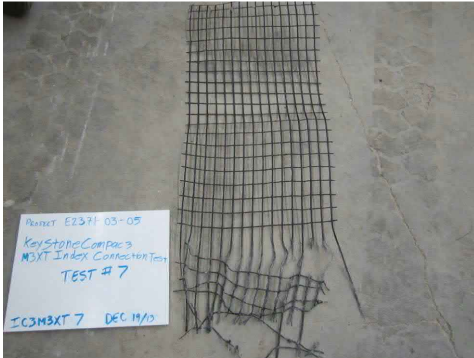
Figure 12: Photograph of the exhumed grid specimen from Test 7.
